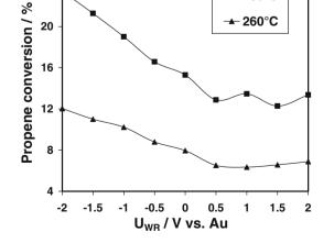
Fig. 3 Influence of the polarization on the propene conversion for Pt/ YSZ at low temperatures. Feed composition: O<sub>2</sub>/C<sub>3</sub>H<sub>6</sub>: 10%/ 1,800 ppm
