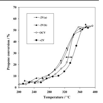
Fig. 1 Propene conversion variations versus temperature recorded after different polarizations during the cooling down process (OCV, -2 V, +2 V). Feed composition:  $O_2/C_3H_6$ : 10%/1,800 ppm
