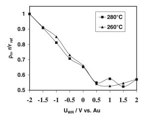
Fig. 4 Influence of the polarizations on the normalized rate enhancement ratio ( $\rho_n$ ) for Pt-YSZ at low temperatures. Feed composition: O<sub>2</sub>/C<sub>3</sub>H<sub>6</sub>: 10%/1,800 ppm
