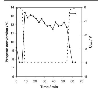
Fig. 2 Potentiostatic transient experiment at 260 °C upon  $U_{WR} =$ -4 V. Feed composition: O2/C3H6: 10%/1,800 ppm
